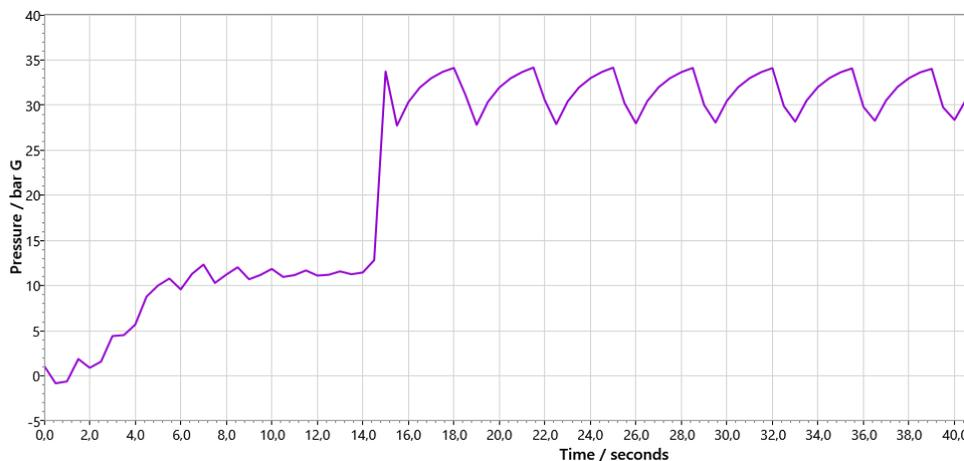
In case of a plant protected by a release and safety valve, we can observe that the overpressure peaks are
