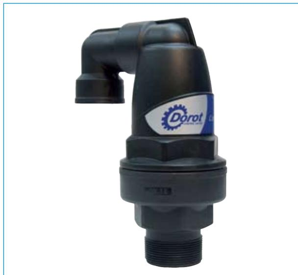
The pressurized air expels the water. The descending water level moves the main float with it. At a certain position the main float pulls down the small seal, that partially opens the nozzle. The pressurized air can escape, the water level rises and the nozzle re-closes.
