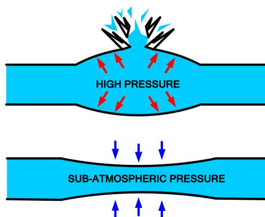
*Note: there are various safety and control devices for limiting water-hammer: surge anticipating valve (RE), pump control valve (BC), deep well valve (DW), two-stage opening valve (TO), quick relief valve (QR), etc. One or more of these may be selected for each hydraulic situation. Dorot has an experienced and respected technical department specialized in studying and resolving water hammer and pressure surge phenomena.*
